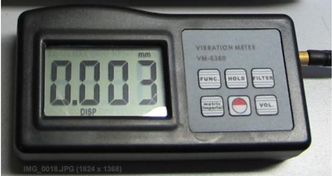
Vibration Meter, VM-6360, measuring mm of displacement.
