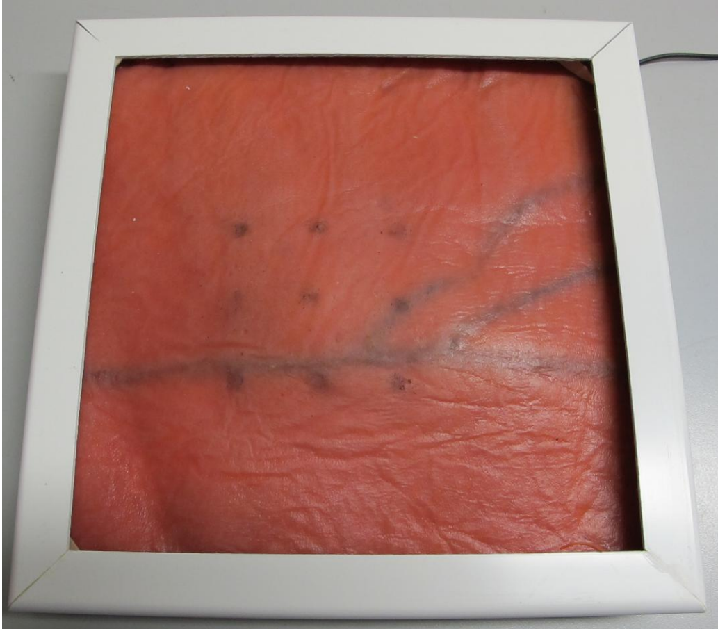
Synthetic Skin Sample, showing the 9 test points.
